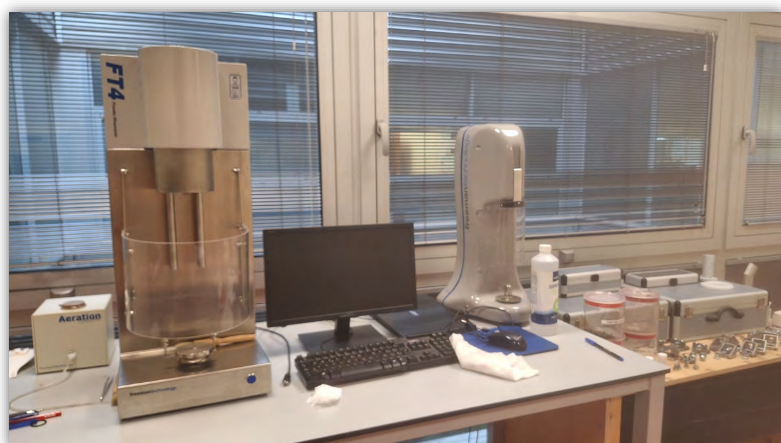
Fig. 2: Silica sand particles (up). FT4 powder rheometer (bottom).
